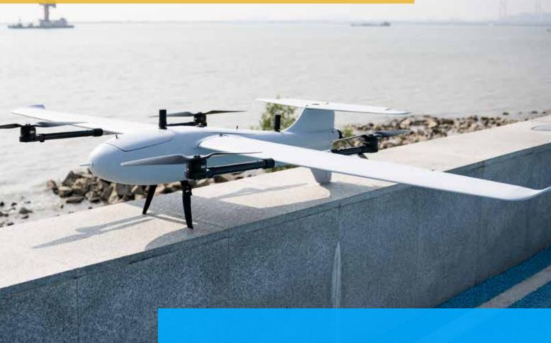
Raefly VT240 is a light electric vertical take-off and landing UAV. The fuselage is made of carbon fiber and Kevlar composite material, which has the characteristics of light weight and high strength. Fluid design, perfect integration of aerodynamics, low flight resistance, battery life up to 4 hours, cruising range up to 260km; detachable design, quick disassembly, reasonable folding and storage design, allowing air transport boxes Smaller size, making operation and transportation more portable
