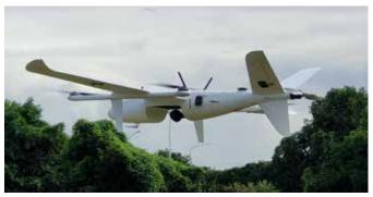
30kg electric VTOL UAV customer tuning case
